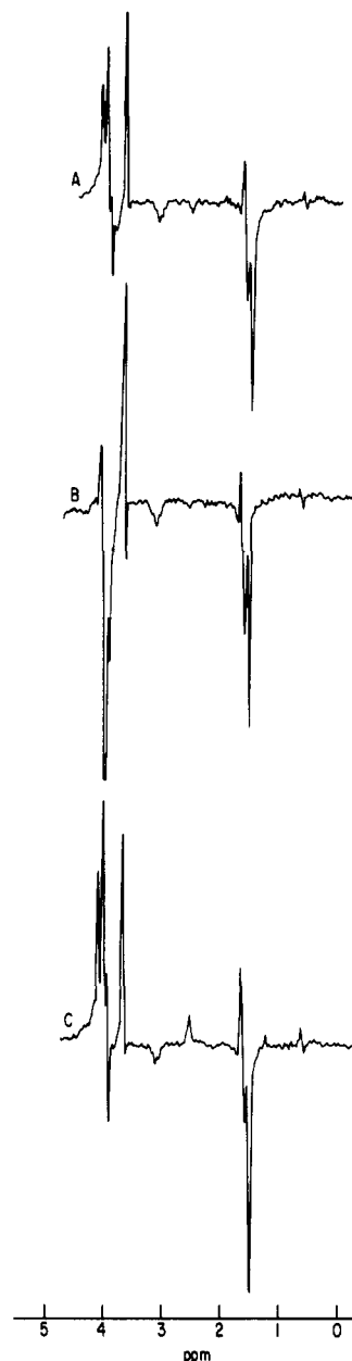
Figure 7. The CIDNP-NR effect in the pulse radiolysis of methanol-methyl iodide in \text{D}_2\text{O} at 1000 G: (A) with electron beam; (B) A with rf at 19.900 MHz; (C) A with rf at 36.500 MHz.
