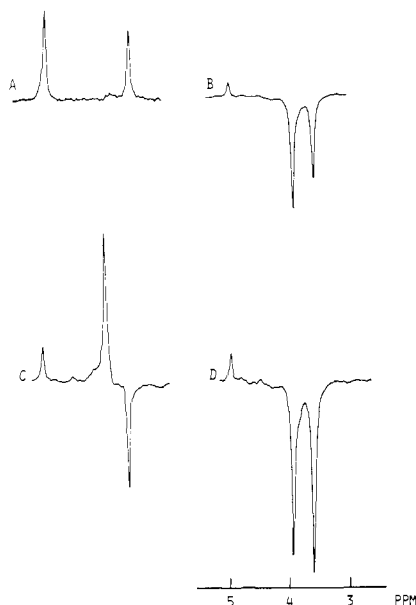
Figure 2. The CIDNP-NR effect in pulse radiolysis of 0.1 M methanol in D_2O at 100 G (methanol, 3.6 ppm; ethylene glycol, 3.9 ppm; HDO, 5.0 ppm): (A) without electron beam; (B) with electron beam; (C) B with rf at 30.000 MHz; (D) B with rf at 23.000 MHz.
